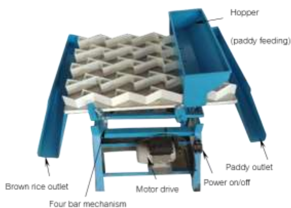
Fig. 1 Compartment-type paddy rice separator machine
