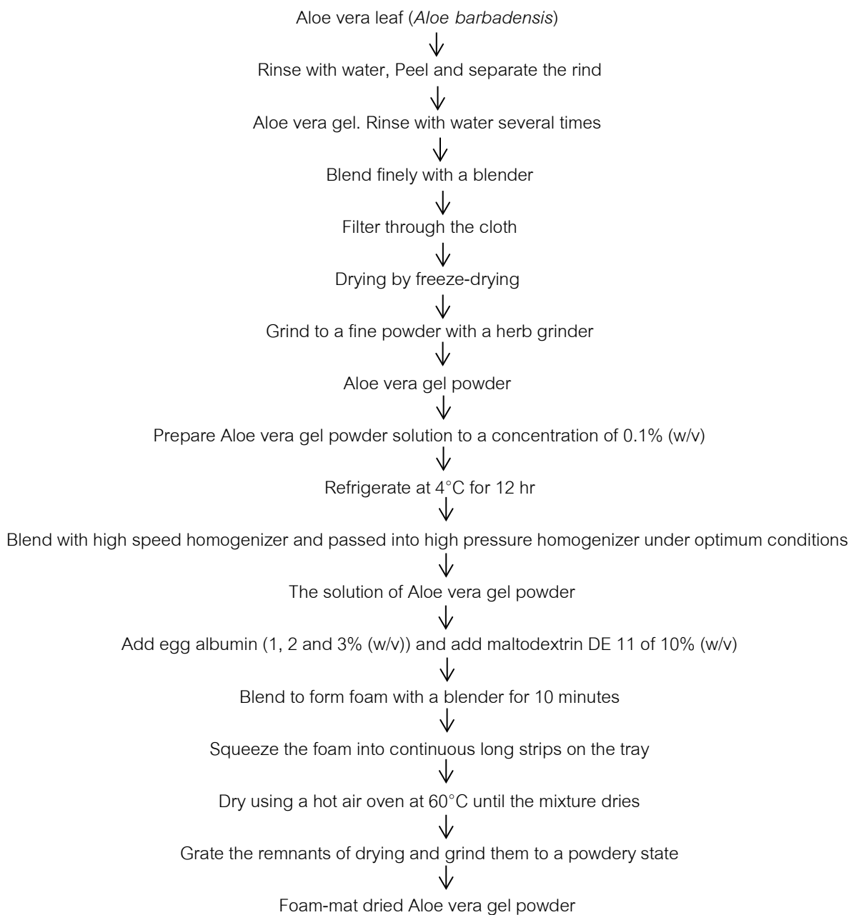
Fig. 1 The process of preparing foam-mat dried Aloe vera gel powder
