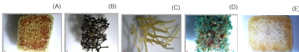
Fig. 3 The stereo microscope observation of the carrier samples in the system after 30 days: Fine PU sponge (A); Coarse PU sponge(B); Loofah (C); Scotch Brite (D); Melamine sponge (E)
