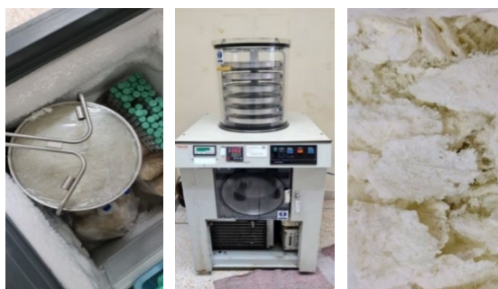
Fig. 2 Preparation of dried Aloe vera gel by freeze-drying method
