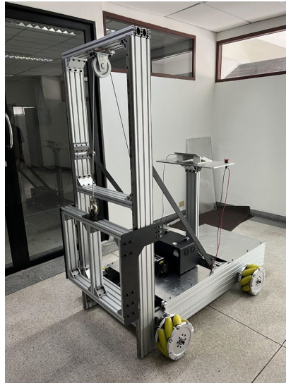
Fig. 2 Forklift made by aluminium profile
